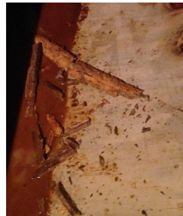
Figure 5: Sloughed Rod Material on Tank Bottom
