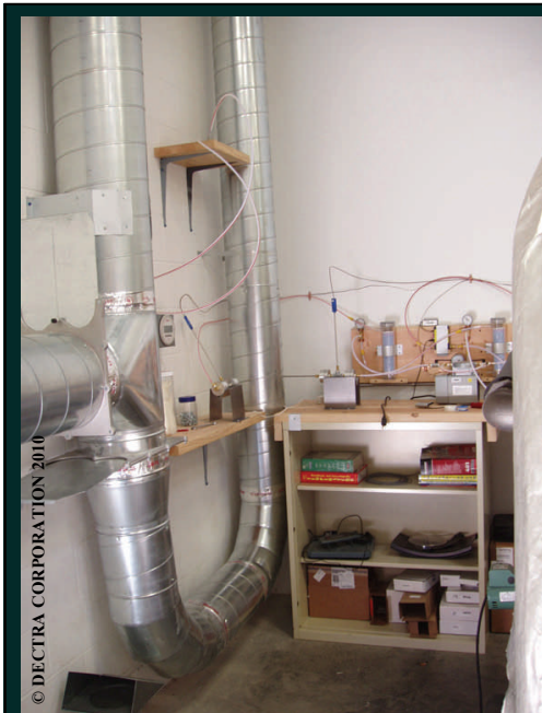
The vacuum pumps, dryer columns, filter housings, gages, thermocouples, flow meters, etc. required for testing. Additional thermocouple wiring and vacuum line work remain. The existing computer system is being utilized for data collection and analysis with this new equipment. The test setup should be complete and debugged shortly.
