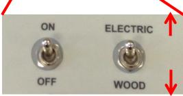
ELECTRIC MODE: Unit may be fired with wood, but it will also use electric for heating if available. If offpeak heating is available it will heat the unit according to the dial switch set point.
