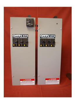
This 33 kW heating package is made up of two (2) 16.5 kW sequencers wired together. The LTDR is mounted on the upper right face of the first sequencer enclosure and can be seen as the small black square.
