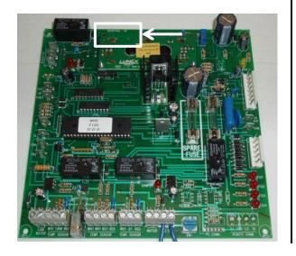
Revision UPC7115**C** or UC7155**D** has the label located here:
