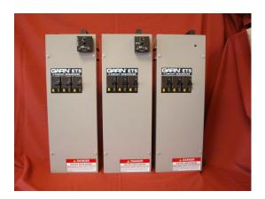
This 49.5 kW heating package is made up of three (3) 16.5 kW sequencers wired together. The LTDRs (2 required) are mounted on the upper right face of the first and second sequencer enclosures, and can be seen as the small black squares in the above photo.
